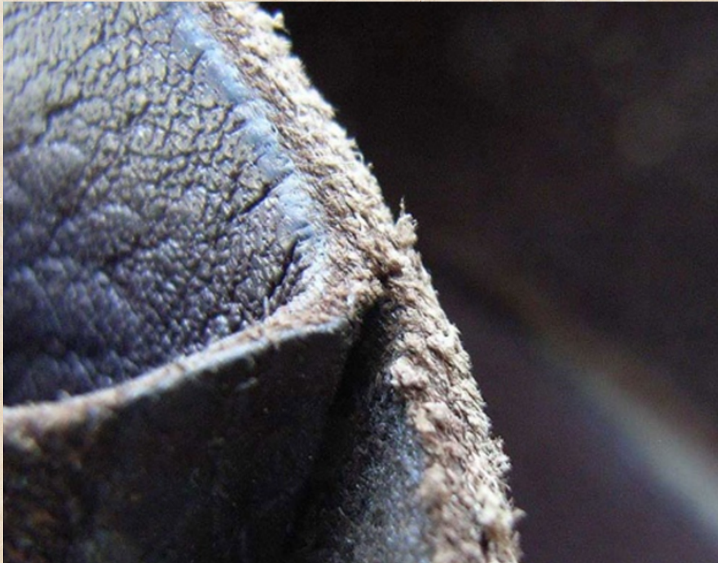
Cow leather is at split into at least two layers
